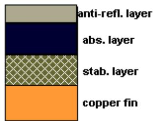
A stabilizing layer of metal is laid on the copper fin. This layer gives the surface of the copper fin long-term stability.
