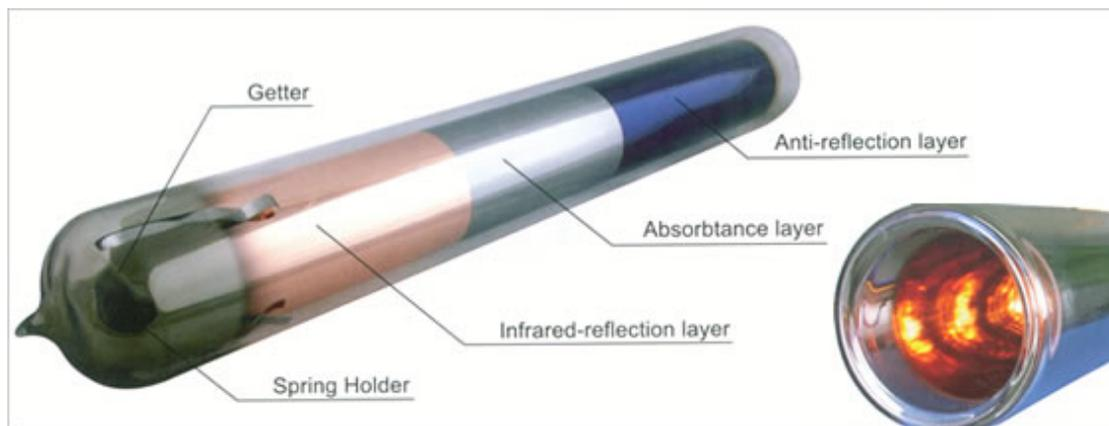
First deposition is a **copper metal** layer, which has low emission ratio and high thermal transmission through inner glass wall to the refrigerant heat pipe.
